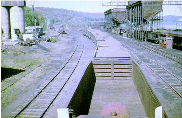
Stamp sand for the Freda mill. A good view of the west end of the Houghton yard in this photo from the top of the diesel looking back at stamp sand cars. This photo, taken in June of 1963 by Charles Sincock, shows a string of rock cars full of stamp sand from the old Atlantic mill at Coles Creek, waiting here for a time before moving to the mill in Freda.
